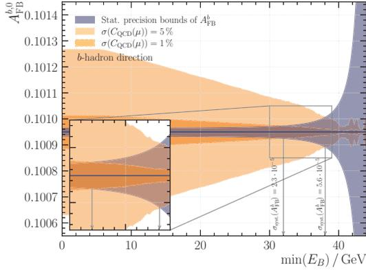
(a) Similar to Fig. 13b, but for the  $b$ -hadron energy instead of the jet-acollinearity on the  $x$  axis, since  $E_B$  does not require to reconstruct and tag the flavour of the jets, which introduce another source of systematic uncertainty.
