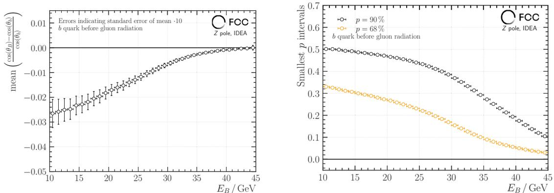
(a) The mean of the relative difference of the  $b$ -quark polar-angle before gluon radiation and the reconstructed  $B$  meson. The uncertainties shown refer to the standard error of the mean and have been scaled by a factor of ten for visibility.
