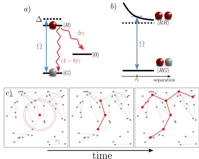
FIG. 1. Overview over the microscopic physics in our model. a) Single atom under external drive  $\Omega$  with decay channels into ground and inactive states. The parameter  $b$  controls the ratio between the decay processes. b) Two atoms with inter-atomic van-der-Waals force that shifts the two-Rydberg state as a function of distance. At  $r = r_f$ , the shift cancels the external detuning and the transition becomes resonant. c) Spreading of an avalanche on a network.
