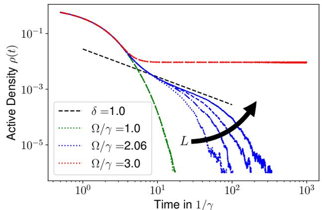
FIG. 11. Finite-size expansion of the active density decay method of finding  $\Omega_c$  for  $v = 10r_f\gamma$ . For all values of  $\Omega$ , we show the averaged decay data for  $L \in \{5, 7, 9\}r_f$ , for  $\Omega/\gamma = 2.06$  we also show  $L = 12r_f$ . The linestyles with increasing system size are: dotted, dash-dotted, dashed, solid.
