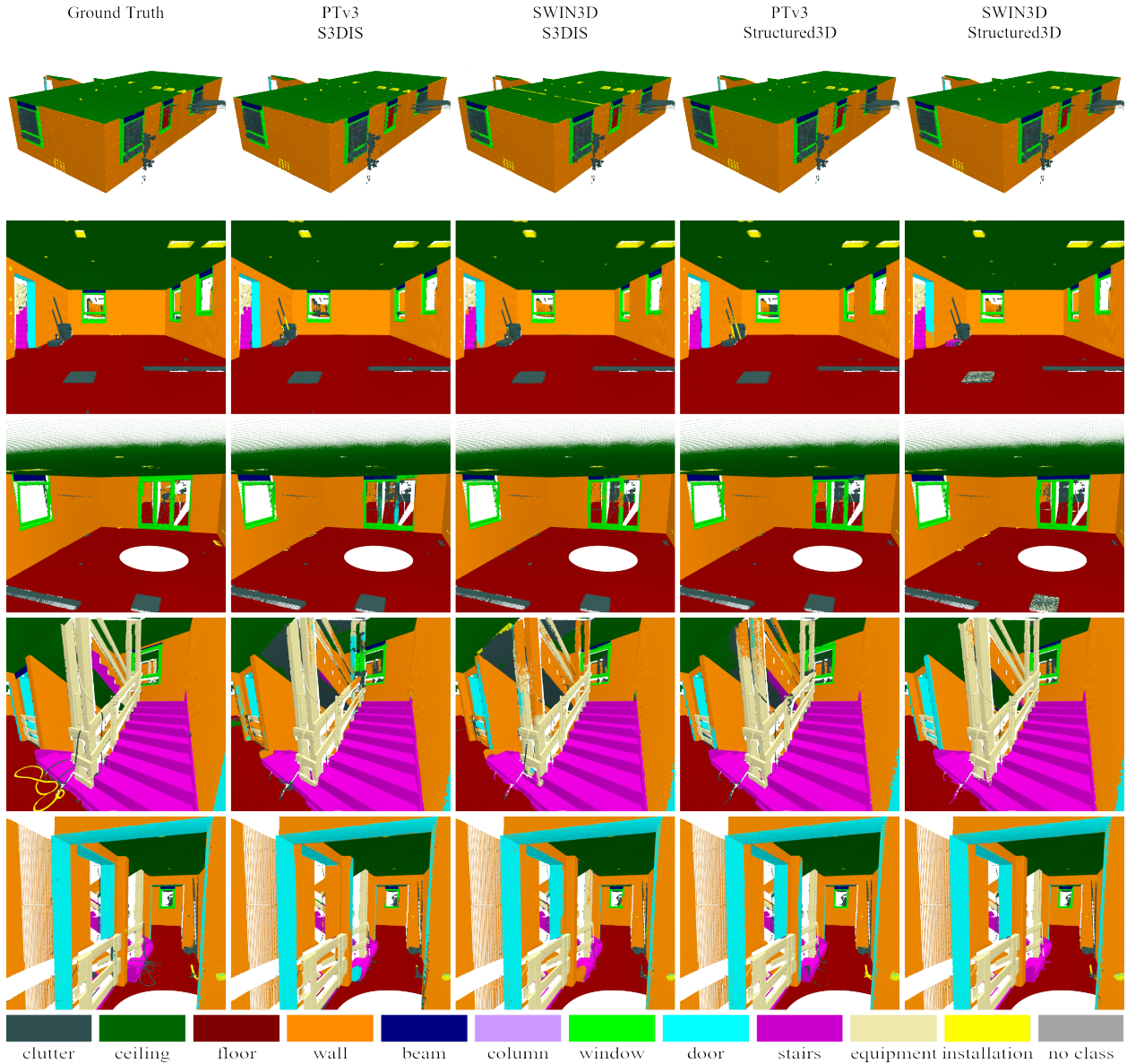
Figure 8: Transfer-Learning Test Results for 3D Semantic Segmentation. This figure presents the inference results from the transfer-learning experiment using two model architectures: Point Transformer V3, and SWIN3D. Each model was pre-trained on one of the two datasets, S3DIS or Structured3D, then further fine-tuned and tested on our custom validation dataset, which focuses on shell construction site scenes. The columns display five representative screenshots per model, with predicted class labels uniquely colored to illustrate the segmentation performance across different architectural components.
