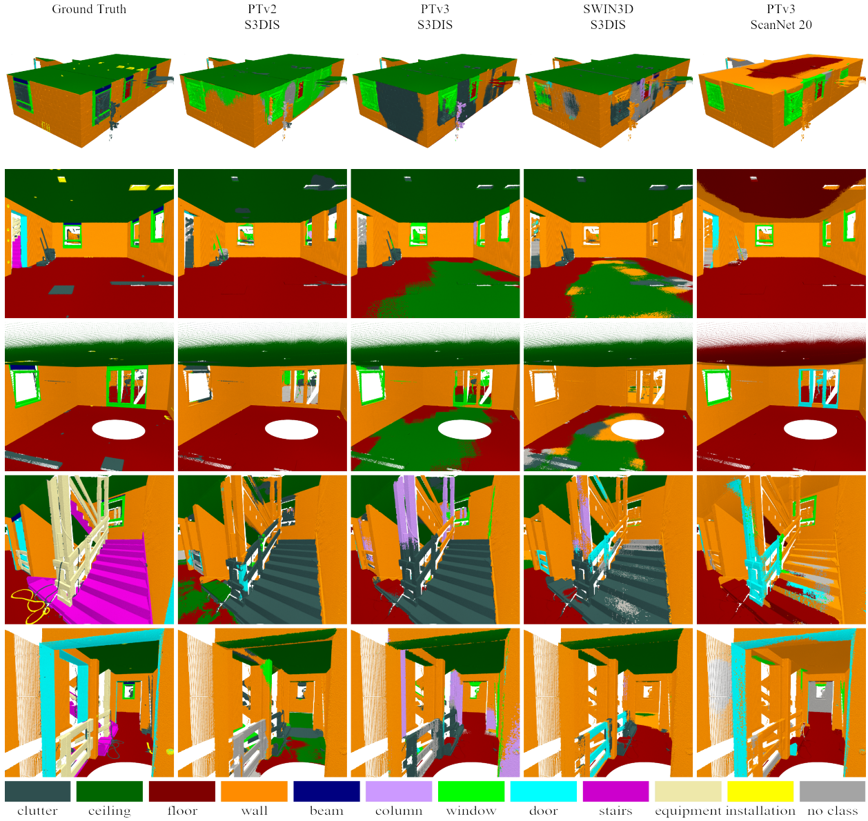
Figure 6: Transfer Test Results for 3D Semantic Segmentation I. This figure presents the inference results from the transfer approach using three model architectures: Point Transformer V2, Point Transformer V3, and SWIN3D. Each model was trained on one of the two datasets, S3DIS or ScanNet 20, and tested on our custom validation dataset, which focuses on shell construction site scenes. The columns display five representative screenshots per model, with predicted class labels uniquely colored to illustrate the segmentation performance across different architectural components. Labels that cannot be translated to one of the 11 target classes, according to the encoding in Figure 1, are assigned to an additional no class .
