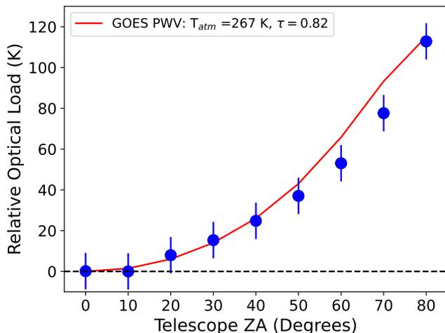
FIG. 13. Top: Measured optical load relative to zenith as a function of telescope ZA. Overlaid in red is the expectation based on the measured atmospheric characteristics from the GOES data and the fyodor analysis package<sup>45</sup>. The agreement is good, indicating that our lab-based calibration model illustrated in Figure 11 accurately describes the KIDs.
