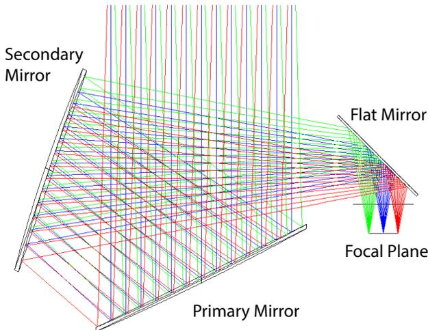
FIG. 5. Ray-trace of the SKIPR telescope optics.
