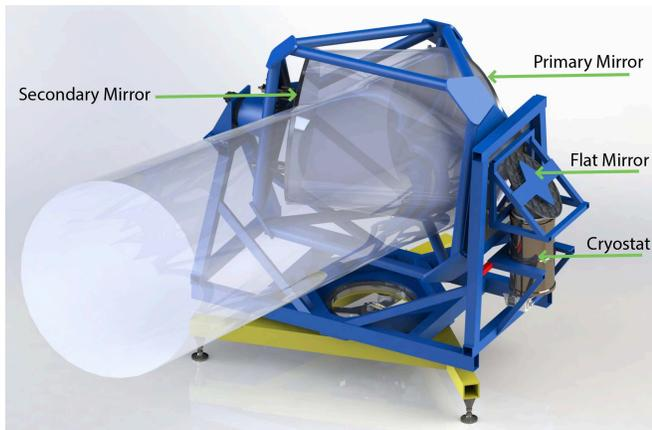
FIG. 1. Isometric view of the solid model of the as-built SKIPR system. The three mirrors are labeled, along with the cryostat that houses the KID FPA at the prime focus of the telescope. A see-through cylindrical solid indicates the optical coupling path to the primary mirror, which is 1.59 m in diameter.
