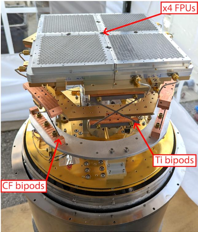
FIG. 3. View of the imager with the cryogenic radiation shields removed. The four focal plane units, each with 960 KIDs, are shown near the top of the image and are connected to the ultracold FAA stage of the ADR. This stage is supported by three sets of Ti bipods connected to the intermediate GGG stage of the ADR. The intermediate stage is in turn supported by three sets of carbon fiber bipods connected to the second stage of the GM cryocooler.
