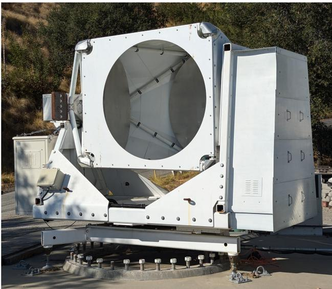
FIG. 6. Photograph of the SKIPR telescope at JPL. The edges of both the primary and secondary mirrors are visible within the circular opening in the baffle structure. The white enclosure to the right of the mirrors is the receiver cabin, which houses the imager cryostat. The total height of the telescope system is approximately 3 m and the total width is approximately 4 m.
