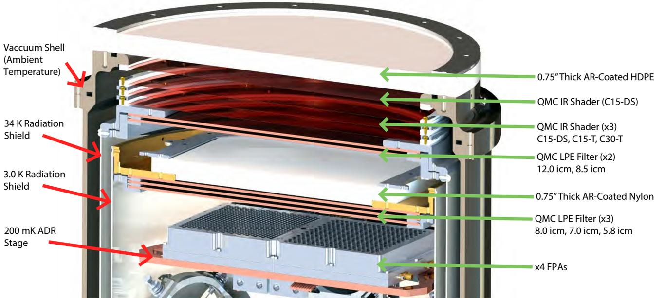
FIG. 2. Cutout view of the optical shaders in the imager cryostat (see Table I for more details).
