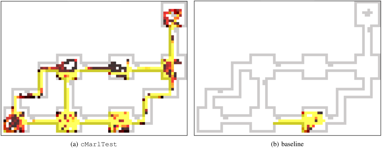
Fig. 3: Spatial coverage for level S1 of Small size. The darker the color the less explored the area.
