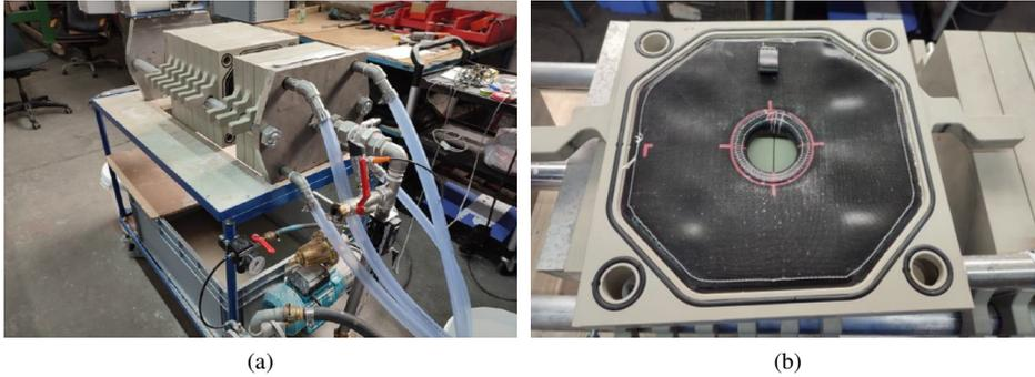
Figure 1: The experimental setup of the chamber filter press, where (a) shows the filter press in its entirety and (b) shows a filter chamber with the filter cloth.
