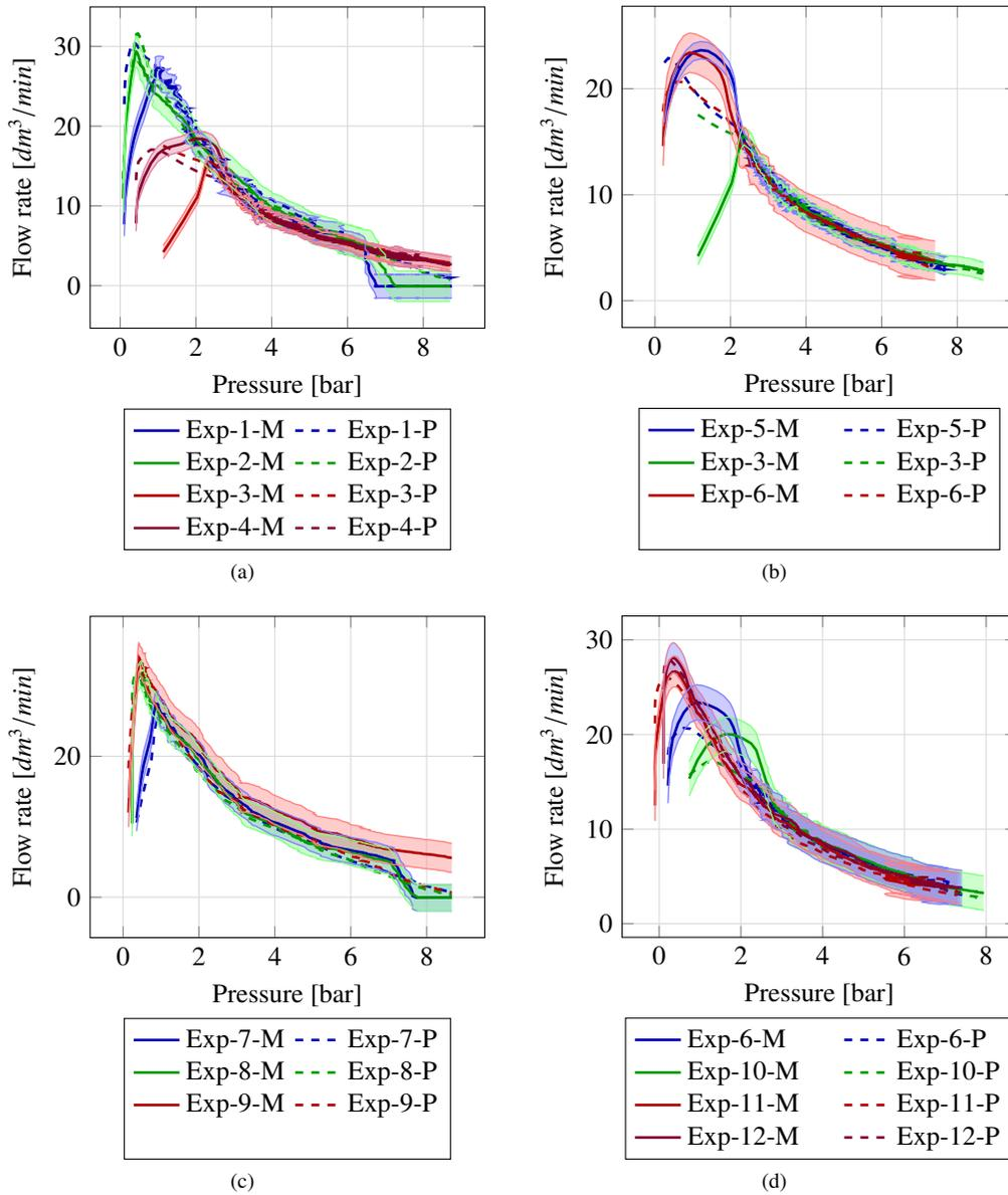
Figure 10: Comparison of measured (M) and predicted (P) flow rate for the experiments from the Table 2. (a) shows the reduction of the flow rate with higher cycle number over the pressure. (b) shows the reduction of the flow rate with different concentrations and similar filter cycles over the pressure. (c) and (d) shows the flow rate with different numbers of filter chambers over the pressure.
