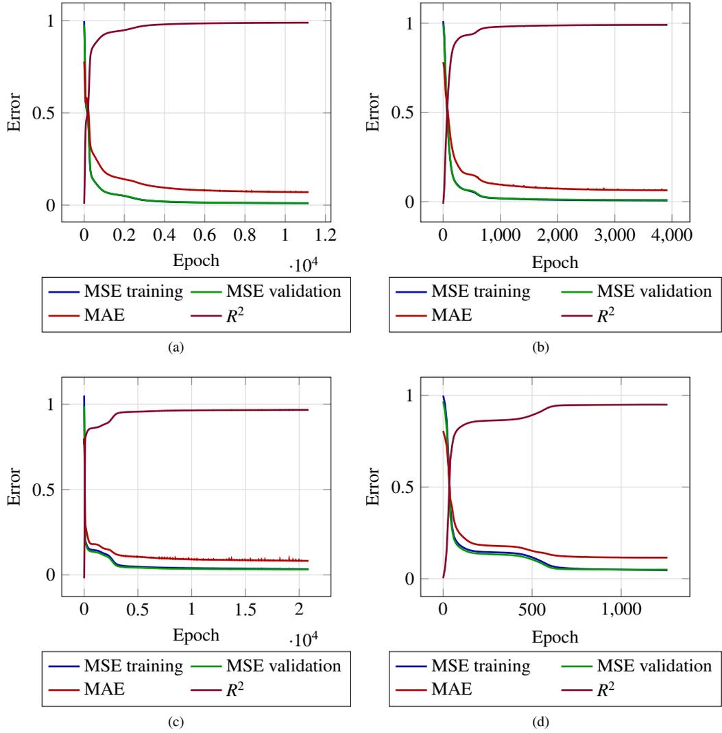
Figure 6: Error metrics MSE, MAE, and R2R2 for training and validation data during training of pressure and flow models. Figure (a) and (b) represent FFNN and RNN models for pressure prediction, respectively, while (c) and (d) depict FFNN and RNN models for flow prediction
