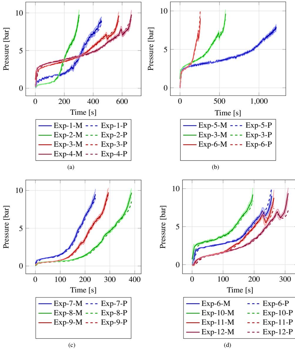
Figure 8: Comparison of measured (M) and predicted (P) pressure values for the experiments from the Table 2. (a) shows the increase of operation time with higher cycle number. (b) shows the increase in operation time with different concentrations and similar filter cycle. (c) and (d) show the operational time with different numbers of filter chambers.
