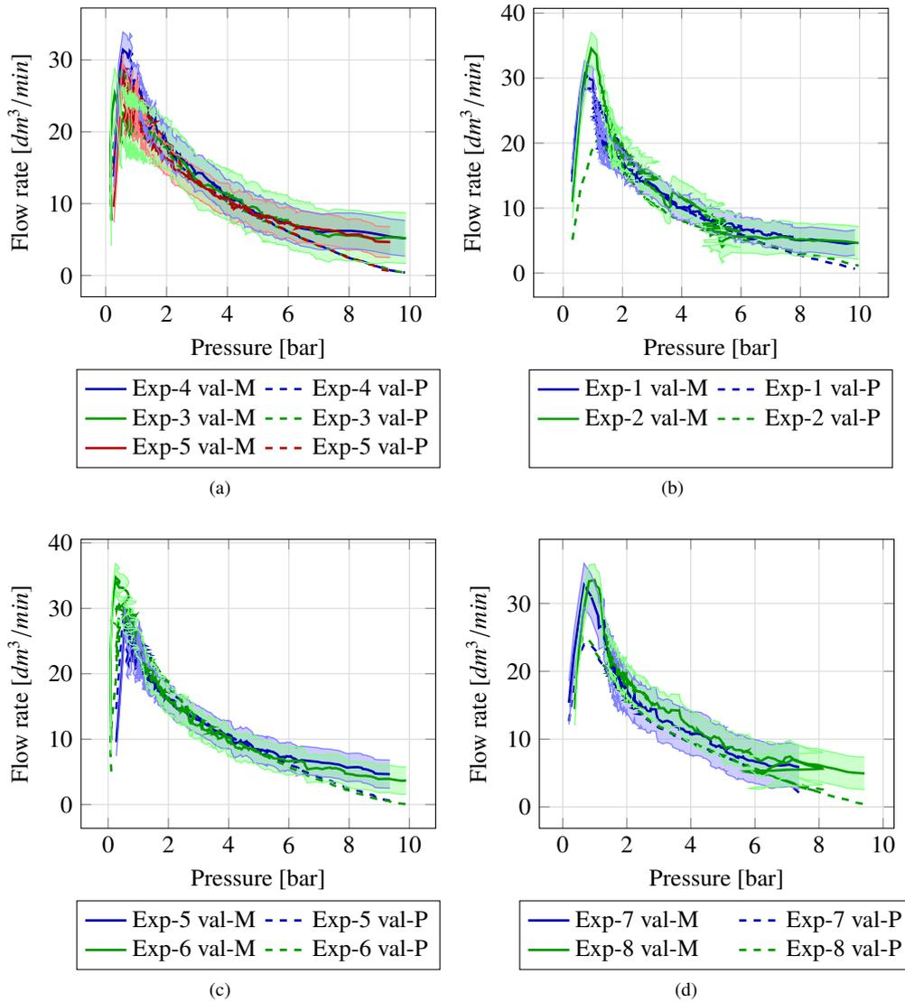
Figure 11: Comparison of measured (M) and predicted (P) flow rate for the experiments listed in Table 3. (a) illustrates the reduction of flow rate with a higher number of filter cycles. (b) shows the reduction of the flow rate with different concentrations and similar filter cycles over the pressure. (c) shows the increase in flow rate with different number of filter chambers. (d) presents the prediction of the flow rate for an unknown concentration of 15 g/L.
