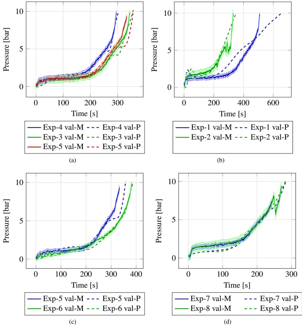
Figure 9: Comparison of measured (**M**) and predicted (**P**) pressure values for the experiments listed in Table 3. (a) illustrates the increase in operational time with a higher number of filter cycles. (b) depicts the increase in operational time for different concentrations while maintaining similar filter cycles. (c) demonstrates the variation in operational time with differing numbers of filter chambers. (d) presents the prediction for an unknown concentration of 15 g/L.
