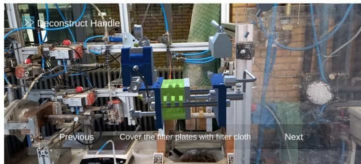
Figure 3: Integration of AR with the DT framework [22]. A three-dimensional model of the chamber filter press is overlaid on the real geometry, demonstrating the potential for visualizing operational states and diagnosing issues such as filter cloth wear or system errors in real time.
