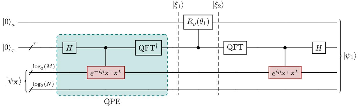
Figure 3: Quantum circuit to prepare the  $|\psi_1\rangle$  quantum state. The red gates represent the parts of the algorithm where the qPCA is implemented, meanwhile, the green part envelopes the implementation of the QPE algorithm.
