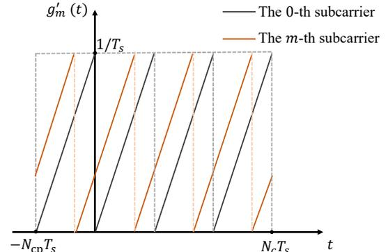
Fig. 2. The frequency of the AFDM subcarriers with respect to time.
