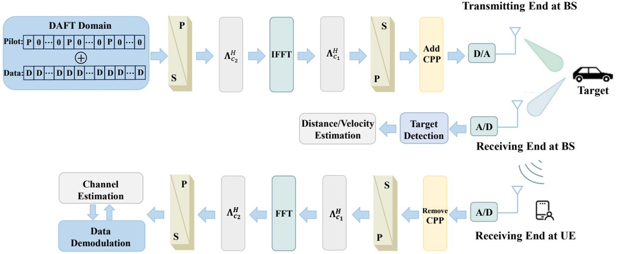
Fig. 3. Transceiver model of the AFDM-enabled ISAC system.
