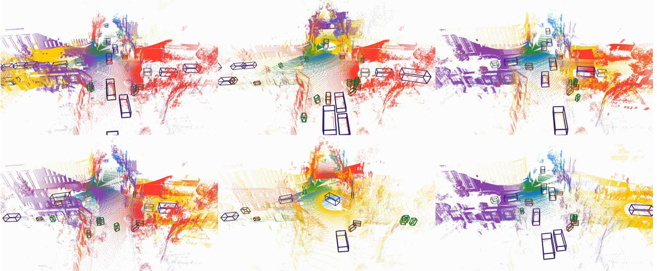
Figure 1. **Six samples of the scenes in the dataset.** The different agent’s LiDAR point clouds are colored according to electric vehicle-001 (EV-1) in purple, electric vehicle-002 (EV-2) in red, urban vehicle (Laser) in yellow, and the RSU DOME and TOP LiDARs are colored in green and blue, respectively. We also draw the annotated bounding boxes within the scene. Best viewed in colour.
