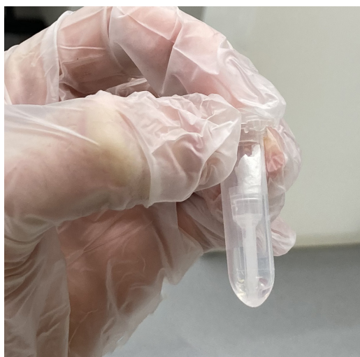
Figure S2: Recovery of electrolytes from aged cells. The glass fiber separator extracted from the cell is placed in a safe-lock tube equipped with a pipette tip. After centrifugation (6000 rpm, 20 min), the electrolyte accumulates at the bottom of the safe-lock tube.
