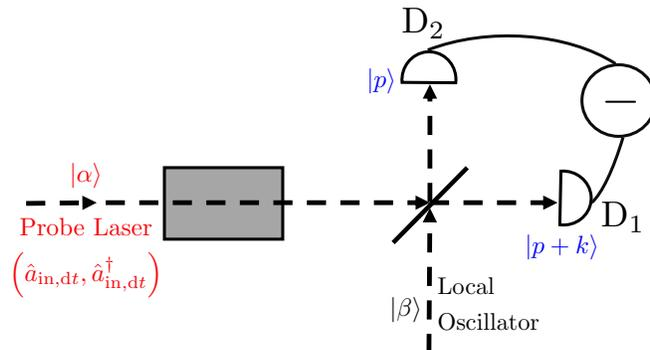
**Figure 2.** In this experimental setup, the gray shaded box represents the cavity, where the strongly interacting Hamiltonian is engineered using cold atoms in optical lattices. The slanted straight line is the 50:50 beam splitter. The two detectors are marked as  $D_1$  and  $D_2$ . This figure has been reused with modifications from Ref. [12].
