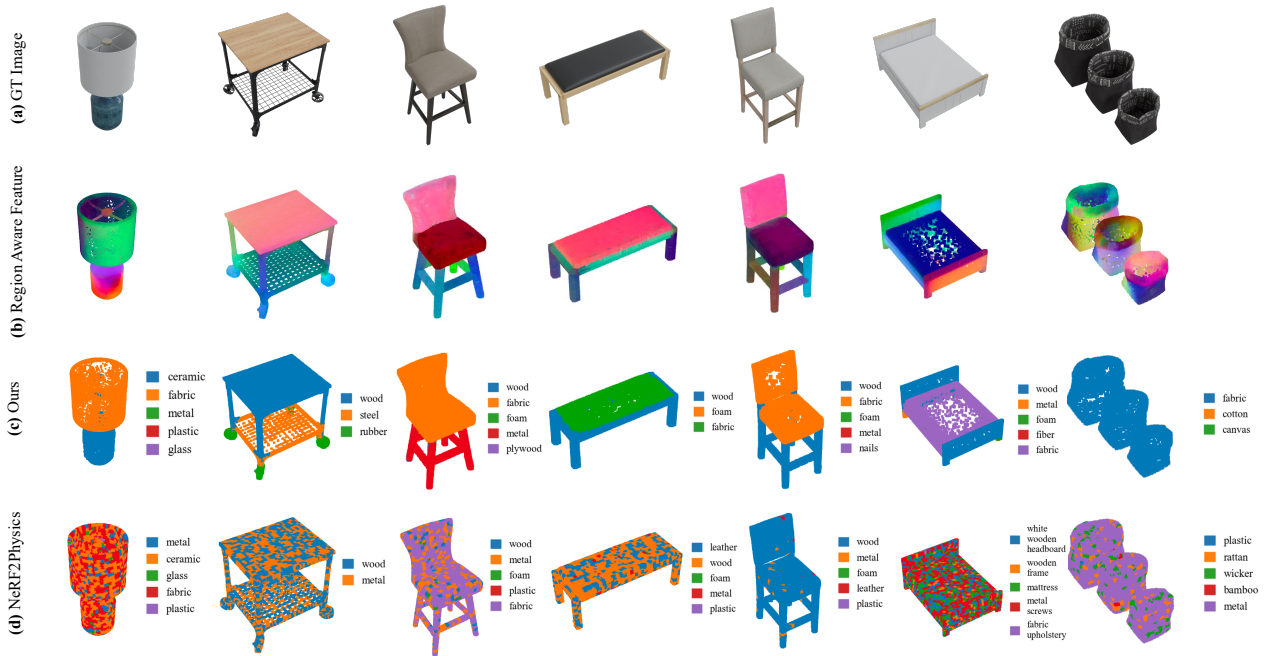
Fig. 5. Region Aware Feature Visualization and Material Segmentation Result of some object. The visualization results in (b) demonstrate that our region-aware feature can effectively identify different regions of the object. (c) and (d) represent the material prediction results of PUGS and NeRF2Physics, respectively. The results from NeRF2Physics are more fragmented, whereas our PUGS achieves more coherent and accurate material segmentation.
