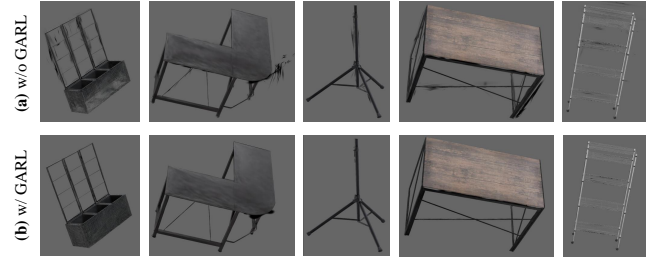
Fig. 3. Comparison of reconstruction results before and after applying geometry-aware regularization loss (GARL). Result (a) without the GARL exhibit some floaters and blurred areas; result (b) with the GARL can achieve the results with more accurate geometry.
