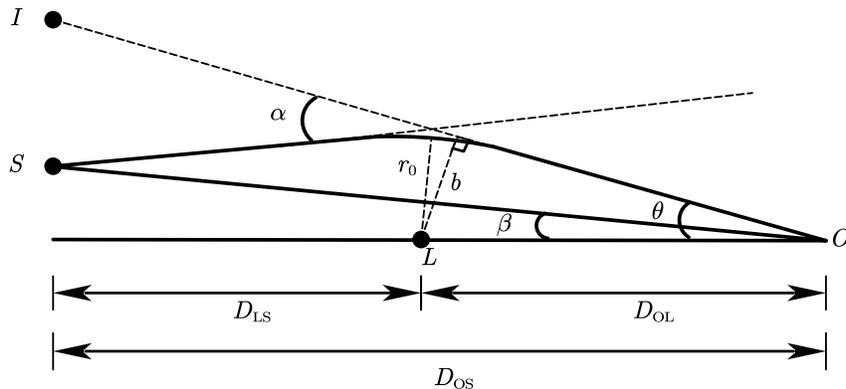
FIG. 1: The fundamental geometric configuration underlying the phenomenon of gravitational lensing.  $b$  is the impact parameter,  $r_0$  represents the minimum distance between the light ray and the lens, and  $I$  and  $L$  denote the positions of the image and the lens.  $S$  and  $O$  represent the source and observer.
