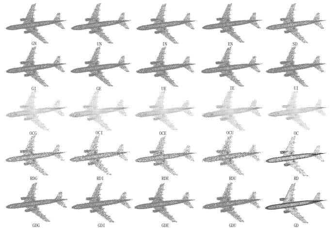
Fig. 2: Snapshots of point clouds degraded by different types of distortions.
