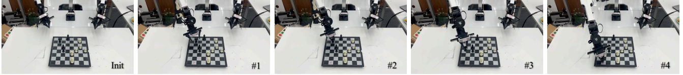
Play Chess : The robot need to Going to Pick (#1), Picking precisely (#2), Moing to target (#3), Targeting (#4). The last image shows it succeeds when the chess piece land on the red-cross position.
