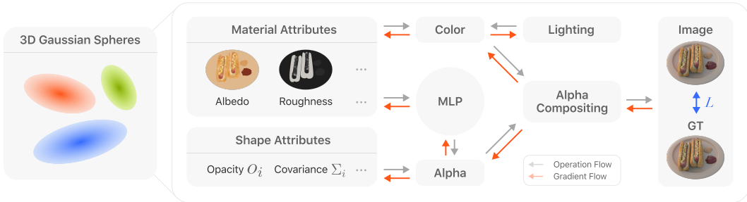
Figure 2: Pipeline overview. We add an additional block to 3DGS-based inverse rendering methods (Liang et al., 2024; Kerbl et al., 2023; Jiang et al., 2024; Gao et al., 2023). Specifically, instead of modeling opacity as a standalone parameter as done by previous works, we augment it against material. By introducing a neural network that takes material properties as input and output cross section and multiplying the opacity with it, we are able to incorporate the Bouguer-Beer-Lambert law into the model. During optimization, material properties not only receive the gradients from color through differentiable PBR, but also the gradients from alpha enforced by the neural network. By doing so, we add an additional constraint to material properties that makes the overall pipeline strictly follow the Bouguer-Beer-Lambert law.
