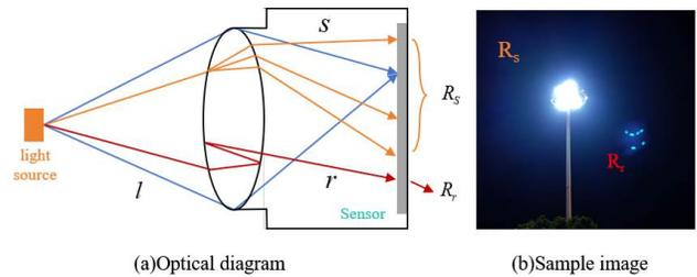
Figure 2: (a) Optical path illustration from the light source to the imaging plane, where the blue line is the ideal light path. The orange line  $s$  is the path of scattered light that produces glow flare  $R_s$ , and the red is the path of light refraction between lenses that produce the reflective flare (ghost)  $R_r$ , and  $l$  is the line of incident light. (b) Example of lens glare.
