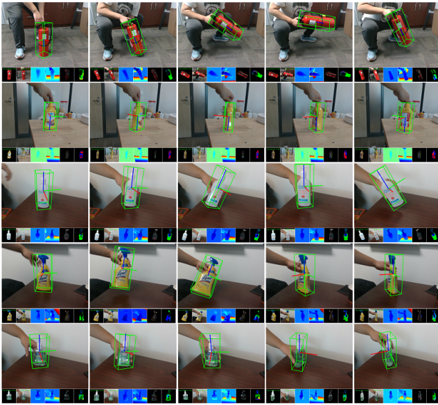
Fig. 12. Demonstration of HIPPO’s zero-shot pose estimation ability. From top to bottom: Fire Extinguisher, Great Value Mustard, Germs Be Gone Sanitizer, Lysol Wipes, and Purell Sanitizer. At the bottom of each image, six sub-images are displayed: rendered RGB, measured RGB, rendered depth, measured depth, RGB residual, and depth residual.
