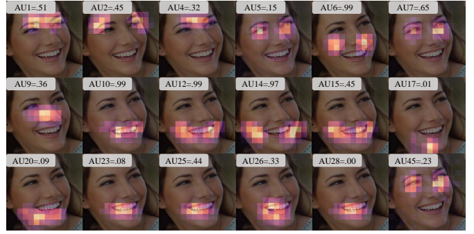
Fig. 6. AGCM offers human-interpretable and intuitive explanations by presenting the contribution of each concept to the prediction alongside its spatial location. The numbers indicate the predicted probability scores for all concepts. During inference, the proposed AGCM generates attention maps for all concepts and assigns probability scores based on the highlighted regions. Concepts with higher probabilities (e.g., AU12) indicate greater contributions to the final label, while concepts with lower probabilities (e.g., AU28) are suppressed by AGCM’s concept generator.
