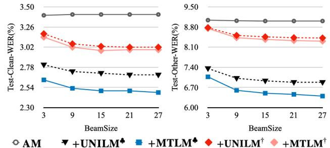
**Fig. 2.** The WER performance of the AM, UNILM and MTLM model when beam size varies. No matter which decoding method is used, MTLM outperforms UNILM and AM. Additionally, the WER decreases regardless of decoding method as beam size increases. Among them, shallow fusion achieves the most significant performance improvement.
