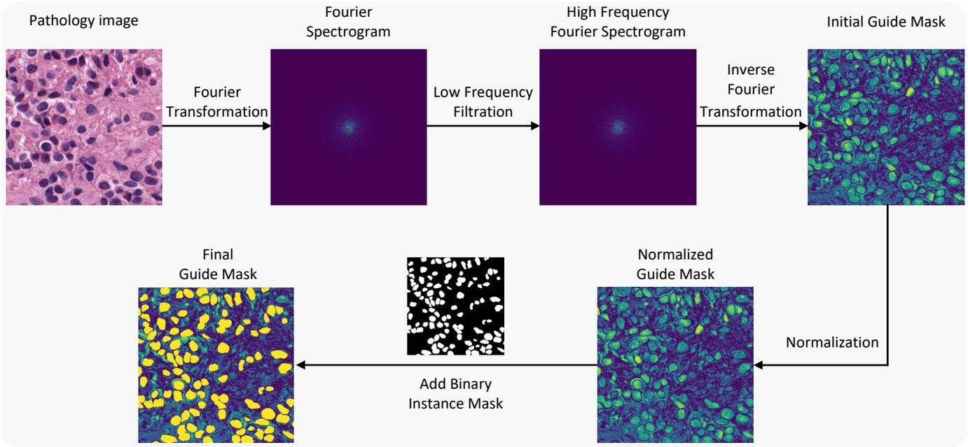
**Fig. 4.** The flow of guide mask generation. For an image, we use fourier transform, low frequency filtering, inverse fourier transform to get the initial guide mask, which is then normalized and added with binary instance ground truth mask to get the final guide mask which is used to guide the model for training.
