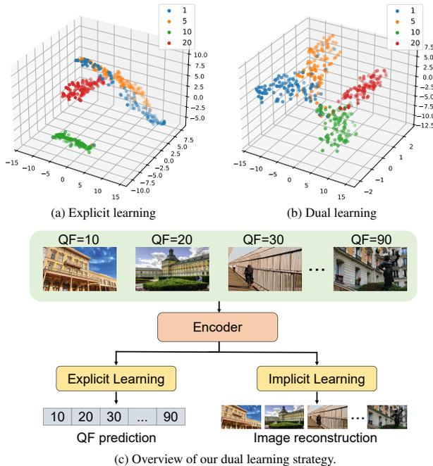
Figure 2. An illustration of the explicit learning approach with our dual learning strategy. We employ the t-SNE [36] method to visualize the clustering of output compression quality representations on the Urban100 [14] dataset, where QF=1 and QF=5 are unseen compression levels. Notably, the explicit learning method struggles to distinguish between these unseen QFs, whereas our dual learning strategy effectively differentiates them.
