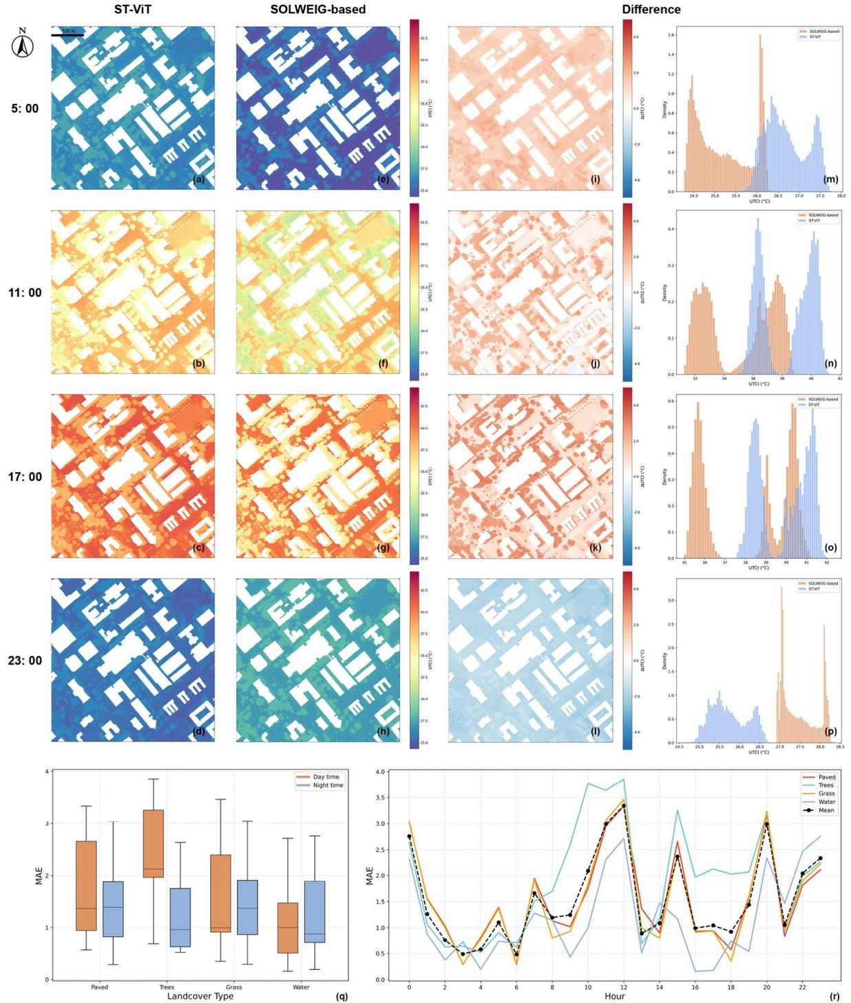
Fig. 3. Diurnal distribution of UTCI predictions from ST-ViT (a-d), SOLWEIG-based simulations (e-h), and their differences (i-p) across typical campus areas ( $500 \times 500$  m) on July 15th, 2022; UTCI prediction errors (MAE) of ST-ViT model (q) during daytime and nighttime, and (r) hourly variation across land cover types.
