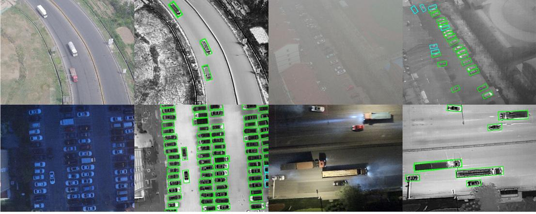
Figure 6: Detection results of our method on DroneVehicle. Green boxes denote true positives; blue boxes denote false positives.
