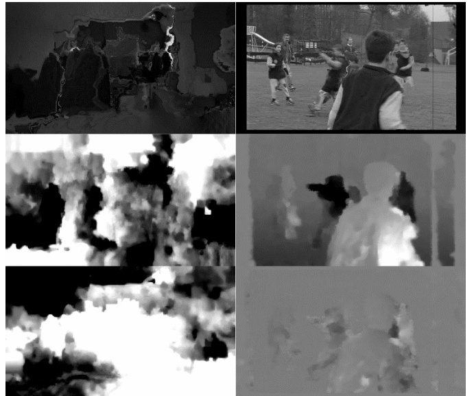
Fig. 1. Left column: warped image and motion field for two frames from different shots. Right column: warped image and motion field for two frames for the same shot. For the motion field, the x-disparity part is visualized in the second row and the y-disparity part in the last row. Disparity is visualized in grayscale (zero value = gray, positive value = white, negative value = black). One can see that the calculated motion field between frames of different shots has large disparity values and is very irregular, and the warped image is very ragged and does not look like normal video content.
