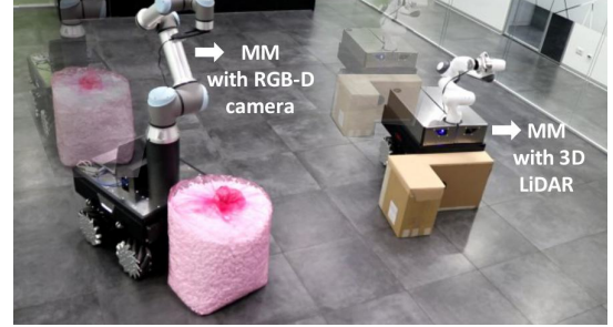
Fig. 1: This study introduces a novel sensor substitution approach that enables non-prehensile manipulation of objects with varying physical characteristics, even when the original sensory information (e.g., contact sensor) used by the mobile manipulators (MM) is unavailable.
