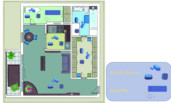
Figure 1: Example Home layout with IOT sensors for monitoring behavioral patterns of People Living with Dementia
