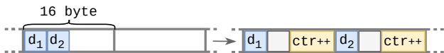
Figure 7: Interleaving counter values and small data chunks in memory. For freshness, the counter is incremented on each memory write. The data chunks are not packed to ease address calculations and elevate stability.
