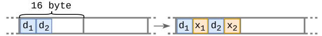
Figure 8: Interleaving data and values for freshness and DMP protection in memory. In order to ensure protection for each 8-byte block in memory, the blocks are split into two chunks of 4 byte each, and contain either data ( d_i ) or freshness and DMP protection values (marked as x_i ).
