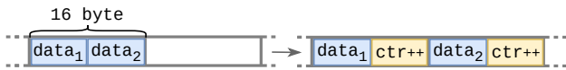
Figure 5: Interleaving data and counter values in memory. In order to ensure freshness in each 16-byte block in memory, the blocks are split into 8-byte counter and 8 byte available for data. On each memory write, the counter value is incremented by one.
