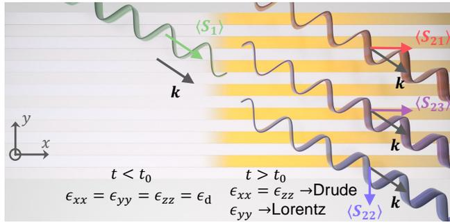
FIG. 1: **Temporal Interface between a simple isotropic medium and a rapidly generated dispersive anisotropic medium:** Different colors of the waves indicate different frequencies after temporal jump.  $\langle S_1 \rangle$ ,  $\langle S_{21} \rangle$ ,  $\langle S_{22} \rangle$ ,  $\langle S_{23} \rangle$  denote the time-average Poynting vectors of the corresponding FW waves. We do also have time-average Poynting vector for the BW waves (not shown here for the sake of brevity)
