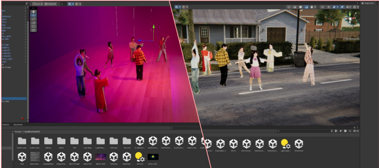
Figure 11. We showcase our custom Unity plugin for relightable 4D Gaussian assets. Our relightable 4D Gaussians are CG-friendly, supporting scene and lighting environment editing within Unity.
