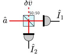
**Fig. S11.** Balanced detection scheme. The input field  $\hat{a}$  is equally divided in a beamsplitter and directed to photodetectors. Vacuum fluctuations ( $\delta\hat{v}$ ) are accounted in the open beamsplitter input. The output photocurrents are given in equations (S19) and (S20).
