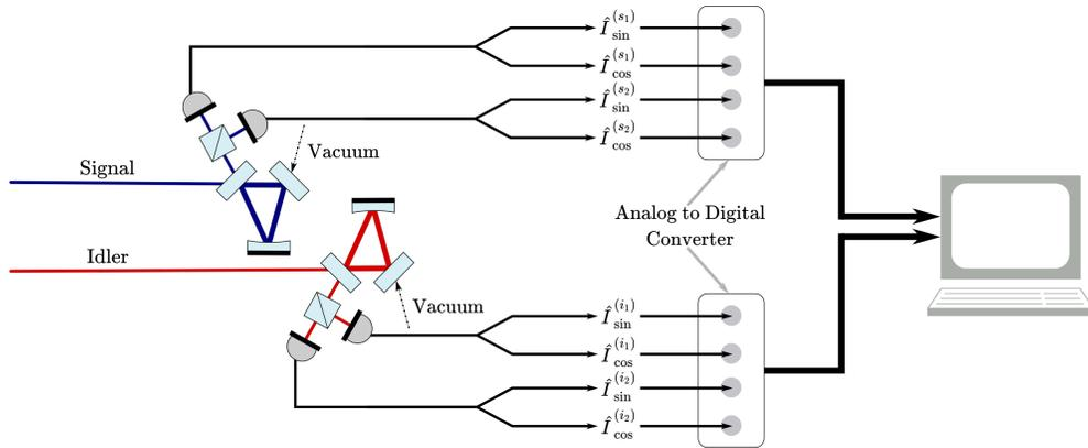
**Fig. S12.** Detection setup scheme. After passing through the resonators, signal and idler undergoes a balanced detection. The double demodulated photocurrents, see figure S1, are individually acquired by analog to digital converters and computationally analyzed.
