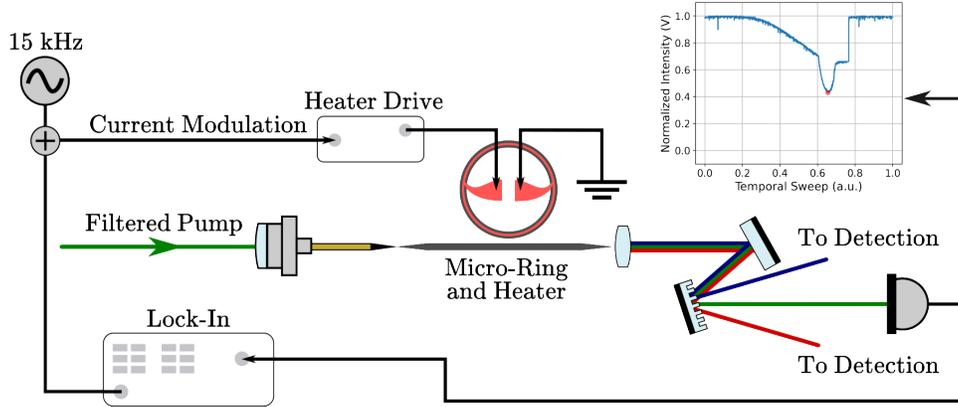
**Fig. S9.** OPO stability system. We modulate the micro-heater at 15 kHz. The separated pump photocurrent is sent to a lock-in system, added to the 15 kHz modulation, to keep the resonant condition stable. The inset shows the separated pump response when a voltage ramp is sent to the microresonator to sweep around resonance. The stability point where we lock the system is indicated by the red dot.
