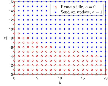
Fig. 3: The structure of the optimal update policy.
