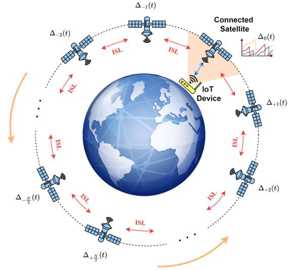
Fig. 1: Status updates from an IoT device to a network of  $(N + 1)$  LEO satellites in an orbital plane.
