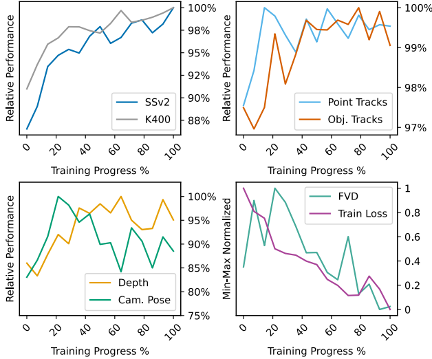
Figure 6. Impact of pre-training progress on downstream task performance – Recognition tasks generally improve with longer training, while tasks like tracking and depth estimation show optimal performance at earlier stages. Performance is evaluated across a range of tasks and compared to training loss and Fréchet Video Distance (FVD).
