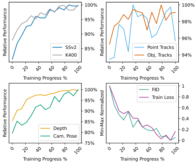
Figure 9. Impact of pre-training progress on downstream task performance of I-WALT – Recognition tasks generally improve with longer training, while tasks like tracking and depth estimation show optimal performance at earlier stages. Performance is evaluated across a range of tasks and compared to training loss and Fréchet Inception Distance (FID).
