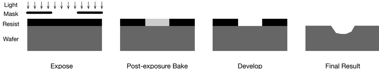
Figure 1. Illustration of a positive resist process.
