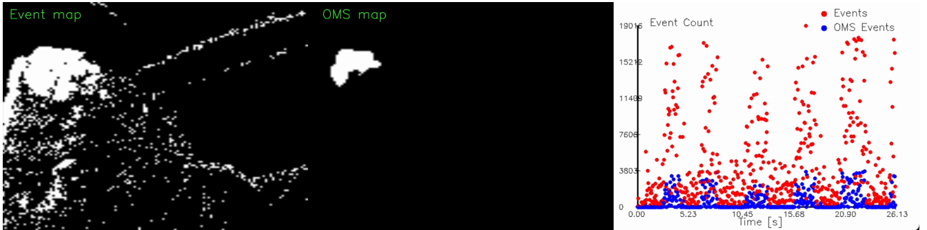
Figure 9: An example from one of the 10 trials illustrating the event counts before and after applying the sOMS model to events received from the DVS sensor ( 128 \times 128 pixels). The events count from the DVS is represented in red and the outgoing events from the sOMS model in blue. The y-axis shows the event count, while the x-axis represents time in seconds.
