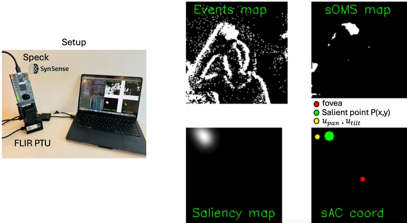
Figure 13: Real-world demonstrator, the Bioinspired attention system. On the left, a view of the setup with the Speck device from SynSense mounted on a FLIR PTU, and the computer displaying the response view. On the right, the response view is shown, including the Events map, the sOMS map, sAC coordinates (where the red dot is the fovea, the green dot is the salient point P(x,y) and the yellow dot sAC commands ( u_{pan} & u_{tilt} ).
