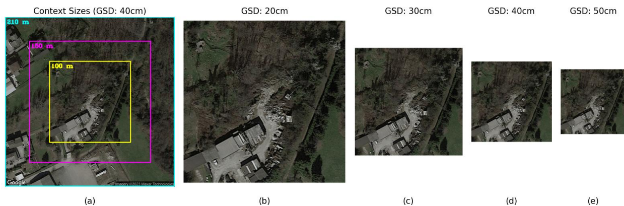
Figure 3: Effects on the Image Size of varying Context Size (a) being equal the GSD, and varying the GSD (b-e) being equal the Context Size (100m)
