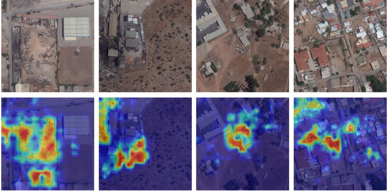
Figure 5: True positive samples with their related saliency maps from the Greek test set used for the generalization experiment. © DigitalGlobe, Inc. (2024), provided by European Space Imaging
