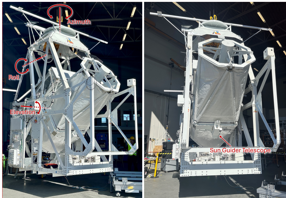
Figure 10. SUNRISE III during the first-light hangtest on May-01 2024 at Esrange, illustrating the gondola Pointing Control System (PCS): The elevation-azimuth actuation, and the roll wheel compensation. The right image shows the location of the Sun Guider Telescope (SGT).
