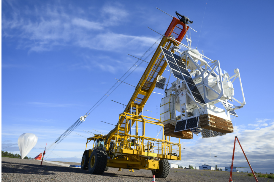
Figure 1. SUNRISE III a few minutes before the launch on July 10 2024 on the balloon pad of Esrange space center. The balloon is already fully inflated, the red and white parachute is attached to the flight train, that stretches over the launch vehicle to the observatory. Image courtesy: SSC / Mattias Forsberg.
