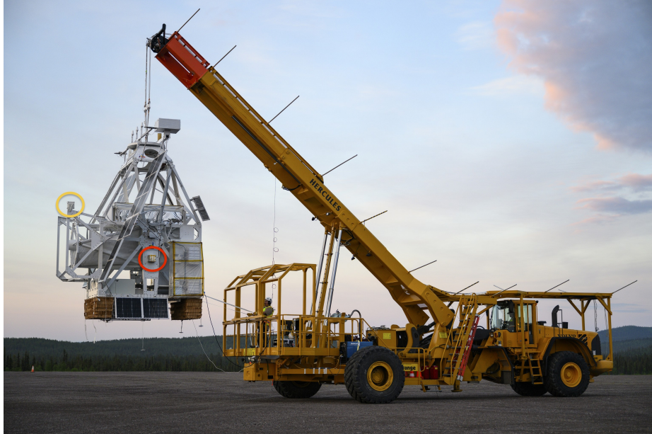
Figure 22. SUNRISE III shortly before the launch on July 10, 2024, hanging on the launch vehicle Hercules. The locations of the piggy back payloads IRIS-2 and RAMON are marked with the yellow and the red circles, respectively. Image courtesy: SSC / Mattias Forsberg.
