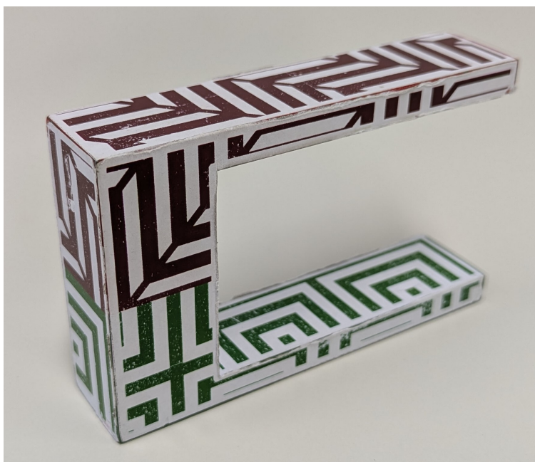
Figure 8: The horseshoe magnet with a particular pattern attached to its surface—for better performance of the object tracking.
