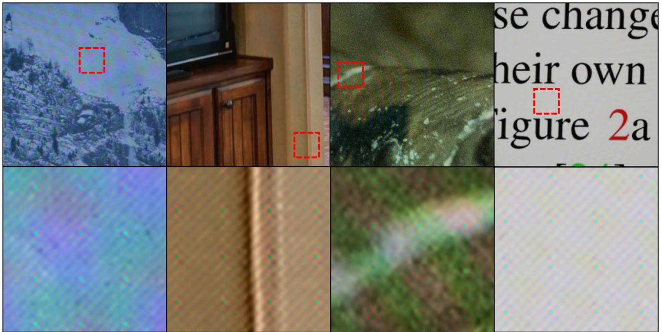
Figure 11: Examples of the “Checkerboard Artifacts” that occur in the I_{trn} when upsampling with Uformer’s transpose convolution (Wang et al. 2022).
