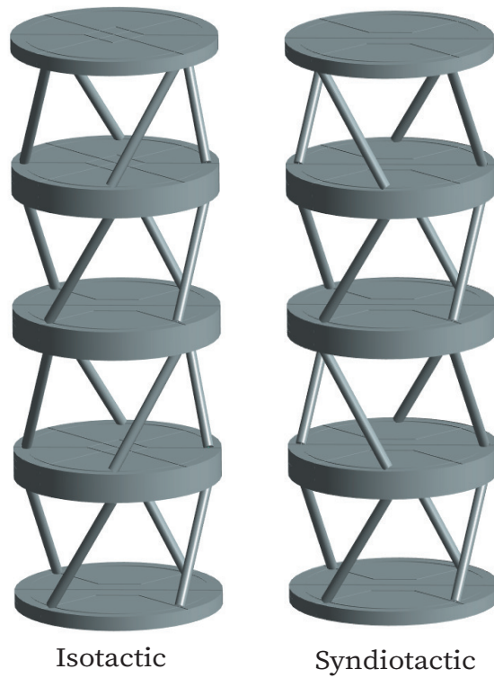
Figure 2: Isotactic (left) and syndiotactic (right) orientations of the chiral links connecting the disks of a chiral phononic crystal.
