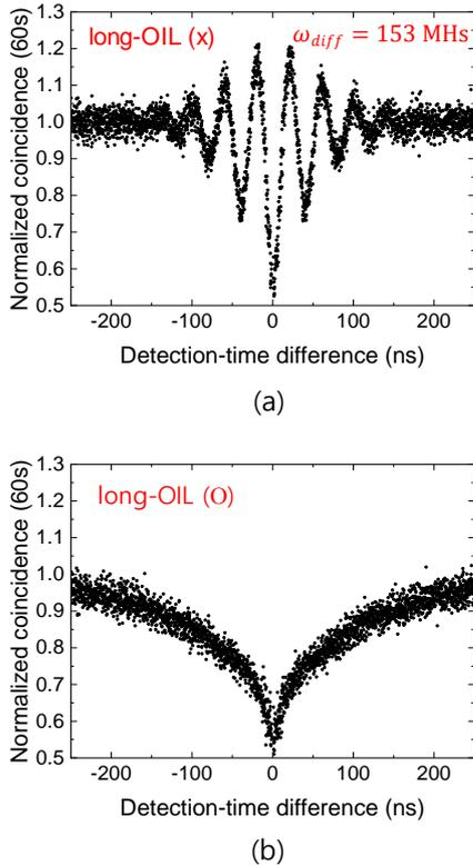
**Figure 4. Time-resolved HOM interference with ICPSs based on long-OIL.** (a) HOM-type two-photon beating fringes under the condition of a frequency difference of  $\omega_{diff} = 153$  MHz between Alice and Bob's optical frequencies without long-OIL. (b) HOM interference fringe with ICPSs after frequency-locking upon applying long-OIL.
