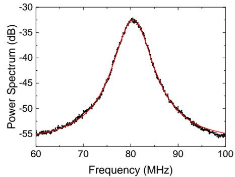
**Figure 2. Frequency-locking via long-OIL.** Beat signal between the frequency-locked Bob slave laser connected via long-OIL with 25 km-long optical fiber and the Alice master laser shifted by an 80 MHz AOM.
