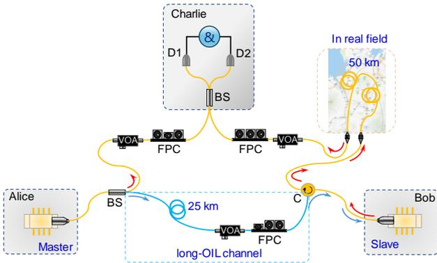
**Figure 1. Experimental configuration for ICPSs based on long-OIL.** ICPSs (Alice and Bob) based on long-OIL and time-resolved HOM interference (Charlie) with two separated CW-mode coherent photon sources with a 50 km-long optical fiber in a real field (BS, beam splitter; D, superconducting nanowire single-photon detector; C, circulator; VOA, variable optical attenuator; FPC, fiber polarization controller).
