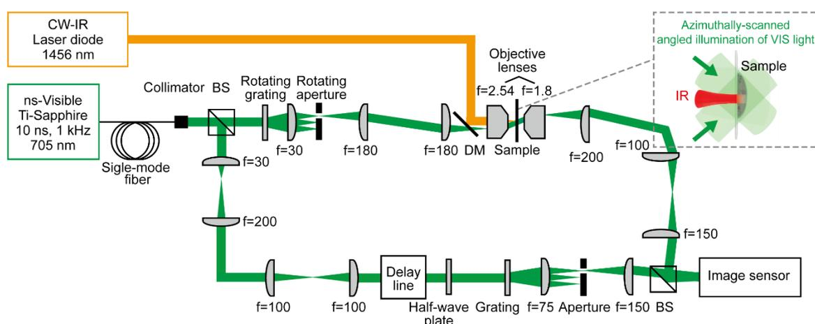
**Fig. S1 Detailed schematic of ViP-ODT.** DM: Dichroic mirror, BS: Beamsplitter.
