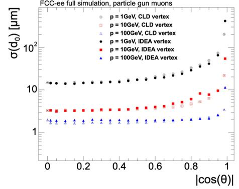
**Figure 2.** Transverse impact parameter resolution in CLD and IDEA VXD [3].
