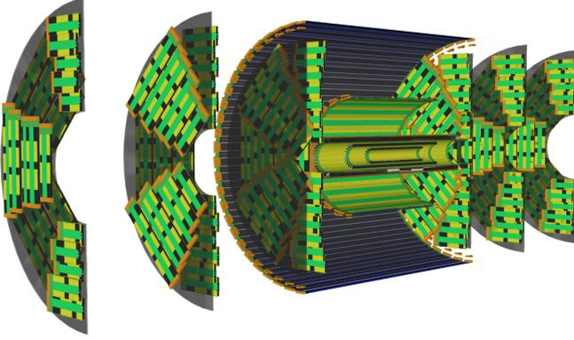
**Figure 1.** IDEA vertex detector full simulation model [3].
