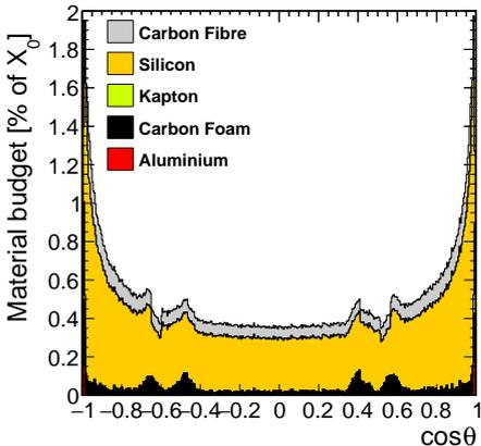
**Figure 4.** Material budget of the four-layer ultra-light inner VXD concept.
