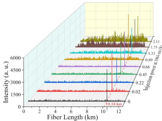
Fig. 3 The vibration localization results of DAS under different delivered power.
