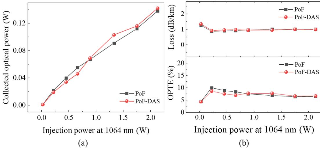
Fig. 2 (a) Collected power of power light, (b) corresponding loss and corresponding OPTE under different injection powers.
