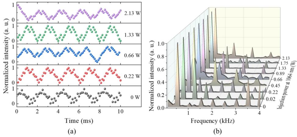
Fig. 4 (a) The demodulation results, and (b) the normalized spectral results of DAS under different delivered power.
