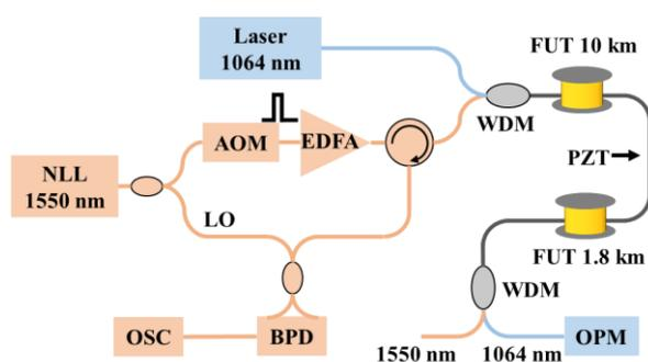
Fig. 1 The experimental setup for the co-transmission systems.
