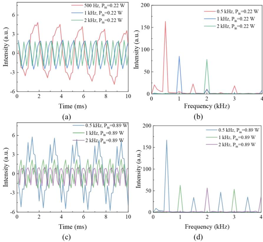
Fig. 5 The demodulation results and the frequency response of DAS at 1064 nm power of 0.22 W and 0.89 W
