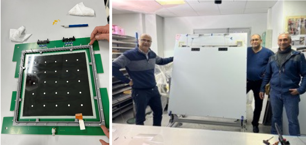
Figure 4: A small, 30 \times 30 \text{ cm}^2 MGRPC with 6 250 \mu\text{m} gaps (left), and a 1 \text{ m}^2 4-gap MGRPC prototype (right), both assembled using the new circular spacer method.
