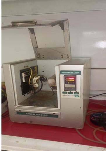
Plate 1: Aerosol Assisted Chemical Vapour Deposition (AACVD) Machine
