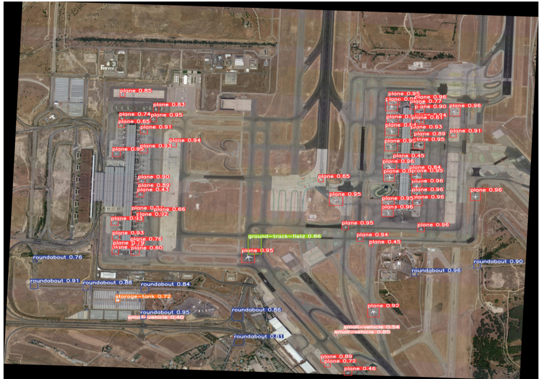
Figure 10. The detection results of the YOLOX model combined with the SAHI framework for the same high-resolution image.
