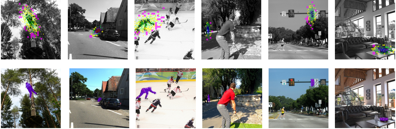
Figure 6. Examples of multi-resolution patch inputs (top row) and corresponding mask predictions (bottom row) from FLIP. Input patches are color-coded by size: purple ( 16 \times 16 ), yellow ( 8 \times 8 ), green ( 4 \times 4 ), blue ( 2 \times 2 ), and red ( 1 \times 1 ). Higher-resolution patches focus on object centers for detail, while lower-resolution patches cover peripheral regions for efficiency. Mask predictions show accurate segmentation with optimized resource allocation.
