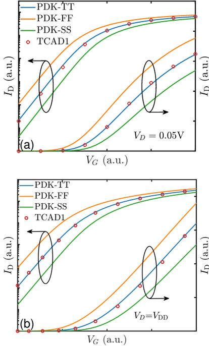
Fig. 2: Calibrated TCAD characteristics of the TT transistor against PDK data: (a)  $V_{DS} = 0.05V$  (b)  $V_{DS} = V_{DD}$ . For comparison the characteristics of the slow-slow (SS) and the fast-fast (FF) corner transistors obtained from the PDK are also plotted.  $T=300K$  (a.u. stands for arbitrary units).
