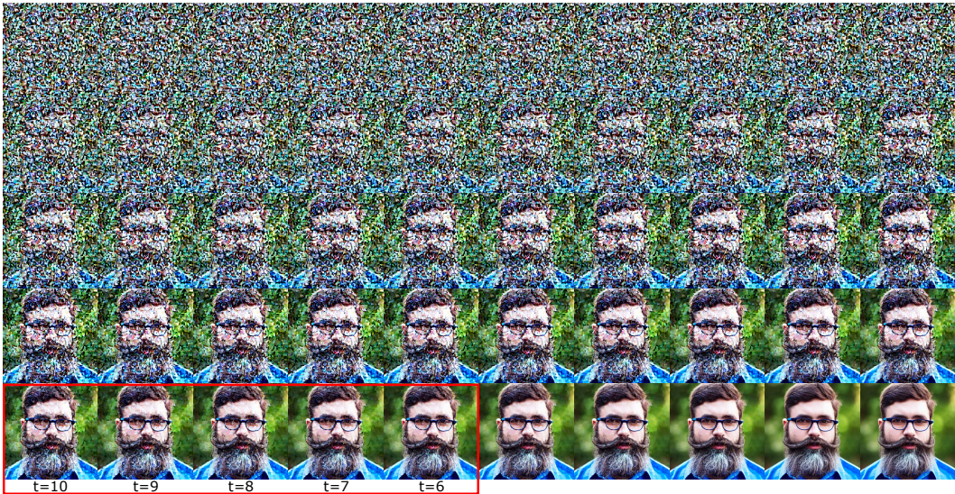
Figure 16: The generated results at each timestep of the diffusion sampling process from T to 1. For example, given one prompt case “A man with a beard wearing glasses in blue shirt”, the noise in the image is gradually reduced from timestep T to 1, and the image is eventually generated with clarity (from left to right, top to bottom).
